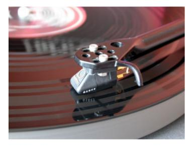
Once you've aligned your cartridge with one of the protractors you are ready to run through the tests. If you are unfamiliar with test records the first thing you will notice are the widely spaced locked grooves; each 'band' contains a different test and you have to cue them individually.
